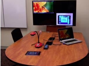
For Instructor operation of the collaborative classroom an iPad is used to provide an intuitive user interface. The instructor can select a podium source or a huddle station to display to the main display and to all of the huddle station.
