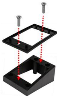
Using the two (2) provided machine screws, attach the back mounting plate to the angled face of the wedge. Ensure that the "↑TOP↑" text on the back mounting plate is facing upwards, and that the arrows point towards the taller end of the wedge.
