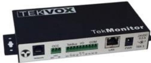
TEKVOX uses Smart Touch Panels that operate the logic of the system. Multiple Smart Touch Panels can easily connect to and be synchronized by TekMonitors using a very simple TCP/IP protocol called TekEzLink. One of the unique features of TekEzLink is to provide device feedback method to all devices connected to it. DSP systems like Tesira also have similar features. This method allows multiple connected Smart Touch Panels to be synchronized without any extra programming.
