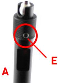
Using a 5/64" hex wrench, tighten the small black screw on the upper black ring of the camera mount stem (A) until snug. **NOTE:** The screw will NOT go all the way in; do not overtighten.
