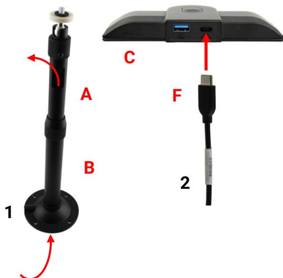
1. Pass USB-C end of USB cable (F, in camera box) up from underneath desk/podium, through camera mount (A/B), and out rectangular cable passthrough hole (oriented away from students in Step 5). *Carefully* feed cable from both ends and work slowly to avoid damaging the cable on sharp metal edges.
