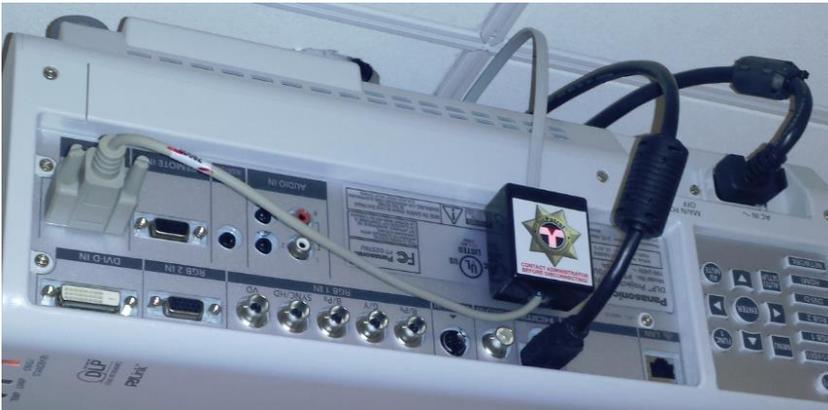
When installing the occupancy sensor it is best to place it behind or above the instructor's and face the vents towards the students. Make certain there are no air vents within 4 feet or air is blowing across the sensor.
