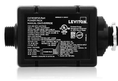
Containing both a 24VDC supply and a 20A line voltage relay for most models, the Leviton compact Power Pack provides low voltage power and line voltage control for Leviton Occupancy Sensors. Versions include Auto-ON and Manual-ON inputs for occupancy sensors, Hold-ON and Hold-OFF capabilities, and a local input for momentary or maintained dry contact switches.
