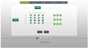
The button matrix displays every possible connection between every input and output, users can carry on the connections by clicking corresponding button.
