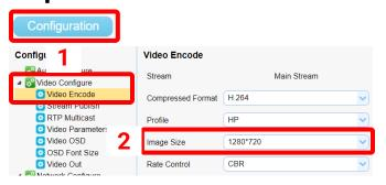
Select the "Configuration" tab at the top of the page, then select "Video Encode" from under "Video Configure" in the list on the left side of the page.
