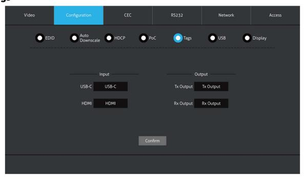
Customize the tags for the HDMI and USB-C inputs, and for the transmitter and receiver HDMI outputs
