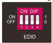
EDID settings for the switcher are controlled by the EDID DIP switches as described below. In the following table, "0" indicates a switch in the Off or Down position, while "1" indicates a switch in the ON or UP position.
