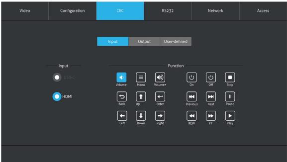
Click a button to send the corresponding CEC command to the device connected to the HDMI input
